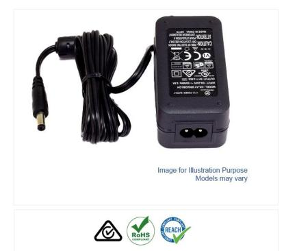
The 25HK-AY-xAz-DH Series is a high-efficiency and standardscompliant 24W External AC/DC Desktop Power Supply. Designed for use in applications such as industrial control and automation systems. This series is supplied with a IEC C8 input connection and supports input voltages of 100~240V AC 47~63Hz.
